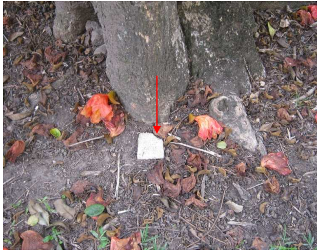
Photograph 21: Accommodation building, Ground level – At the base of the north west side 'African tulip' tree; Asbestos cement sheet fragment.
