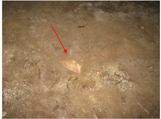
Photograph 22: External: Ground level, Main hall building – Central sub-floor area opposite workshop; Asbestos cement fragments found at ground surface.
