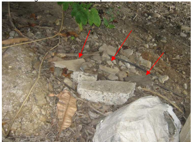
Photograph 19: Accommodation building, Ground level sub-floor area – Below north west side stairs; Asbestos cement fragments. Refer to sample CA7478
