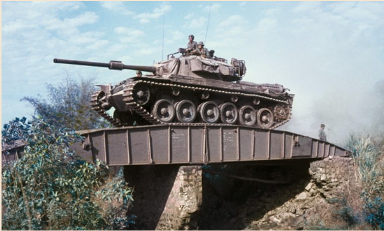
↑ A Centurion Mk V/1 tank crosses a bridge which had been laid by a Centurion bridge layer over the remains of a destroyed bridge just south of Xuyên Mộc, August 1969. (AWM P05873.001; photographer Kenneth Alfred Toccock)
