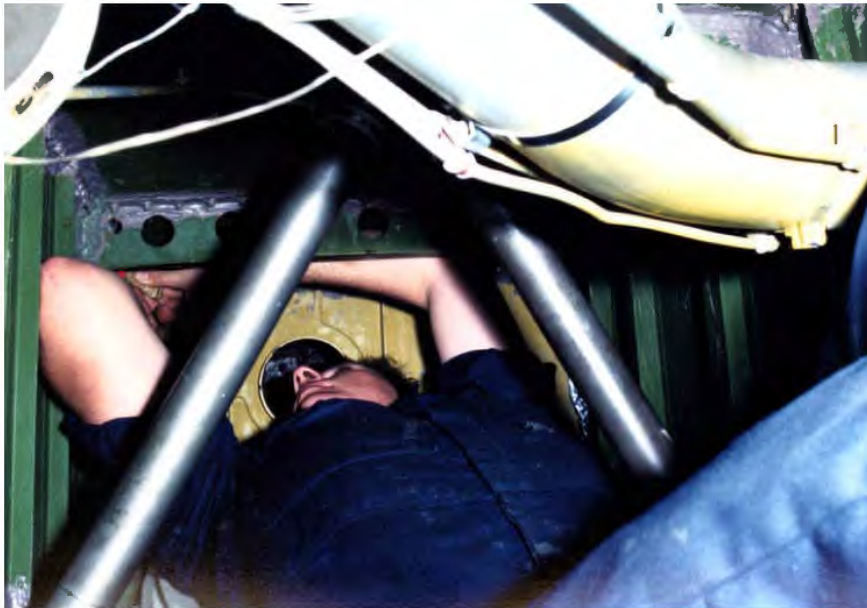
Figure 1.3 : A technician checking sealant in the fuselage tank
