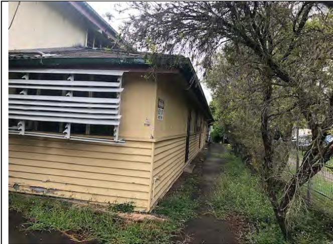
This image shows the Southern elevation along the Headfort St fence line. Scaffolding will be erected to this face to provide a clear barrier delineation between the pedestrian foot path and the work face.
